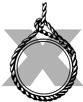
Incorrect – Cutting action of eye splice on running line.
