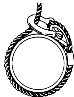
Correct – Shackle pin cannot turn.
