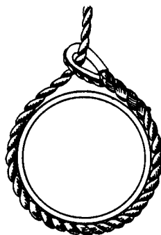
Correct – Use thimbles in the eyes.
