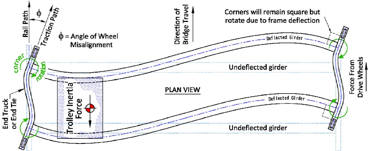
**Figure 1: Bridge Frame Deformation**
